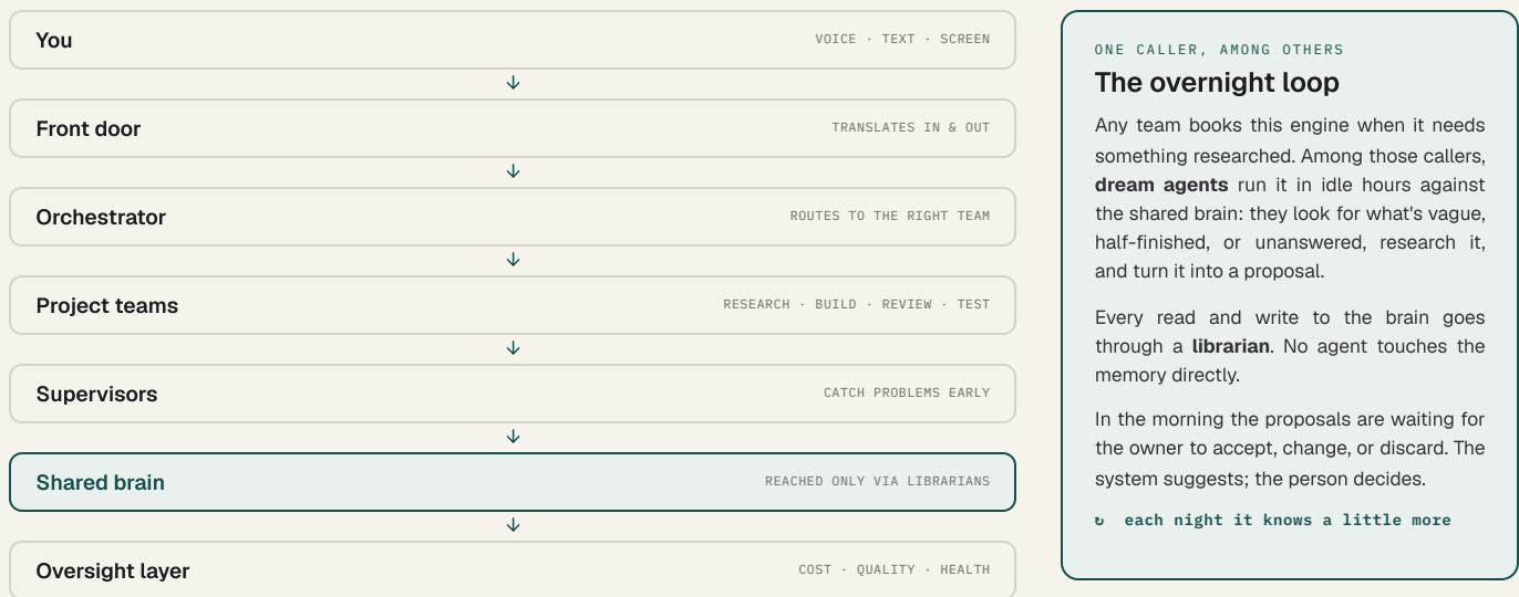
Figure. The engine is reached through librarian agents over the shared brain, under an oversight layer watching cost and quality. The same loop that researches the outside world can be turned inward to research TARS itself, but its only output, on any target, is a proposal that surfaces to the owner.
